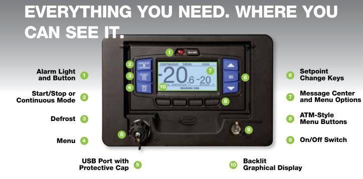
A large dashboard-style display shows all key operating information, providing an at-a-glance visual indicator of both unit operation and conditions inside the trailer.
